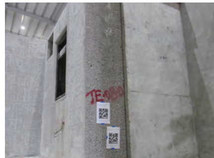
TOP, ABOVE LEFT AND ABOVE: With digitisation at its new ‘smart’ Jurong Port factory, Dragages can monitor the work progress in real time through the use of QR codes.
