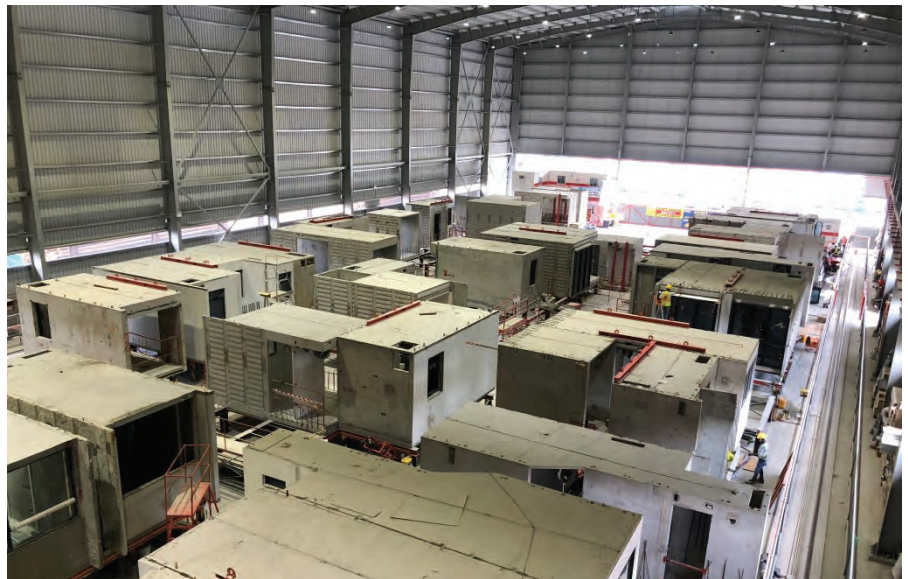
ABOVE, BELOW LEFT AND BELOW RIGHT: PPVC modules for residential projects being stored in Dragages’ new facility at Jurong Port, Singapore. The modules will be completed with internal finishes, fixtures and fittings prior to delivery.
