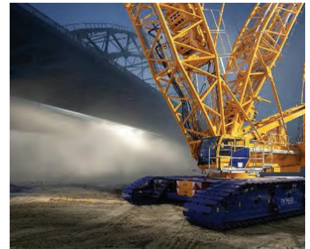
BELOW: Demag CC 2800-2 lattice boom crawler crane.
