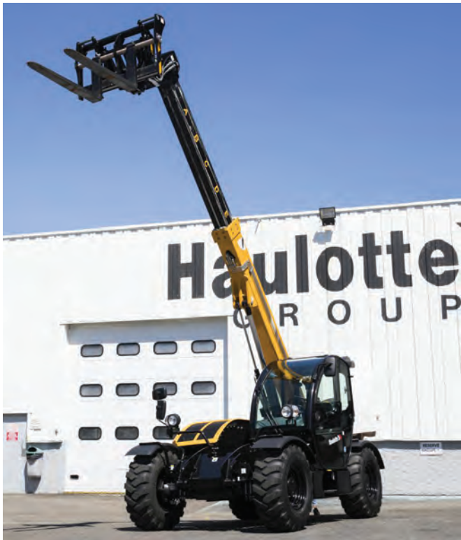
ABOVE AND LEFT: Haulotte's new HTL 3207 telehandler offers a maximum lifting capacity of 3.2 t and maximum lifting height of 6.85 m.
