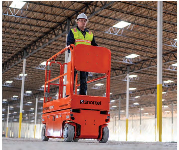
ABOVE AND BELOW LEFT: The Snorkel S3019E scissor lift is equipped with both electric drive and electric steer. The machine can lift up to 250 kg to a maximum platform height of 5.79 m.
