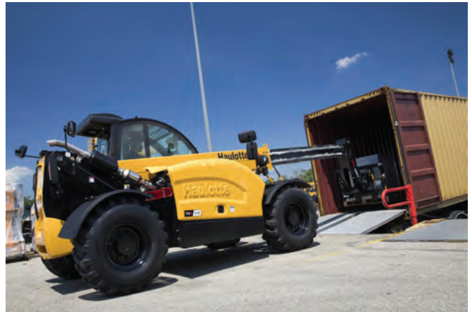
ABOVE AND LEFT: Haulotte's new HTL 3207 telehandler offers a maximum lifting capacity of 3.2 t and maximum lifting height of 6.85 m.
