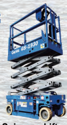
Scissors Lift Working Height (6 - 18 Metres)
