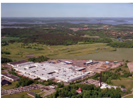
ABOVE LEFT: At the axle and transmission factory, Volvo CE has invested in an energy recovery system that will conserve around 60% of the heat generated in the hardening centre (pictured) and transfer it to paint shop.
